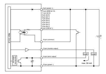
\*The current consumption for pins 1 to 4, 6 to 9, 11, and 12 is approximately 6 mA.
