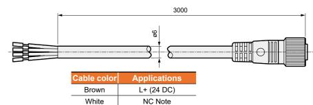
C (IO-Link) Black Note: Insulate so that there is no contact with other wires.
