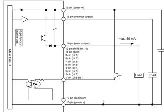
\*The current consumption for pins 1 to 4, 6 to 9, 11, and 12 is approximately 6 mA.
