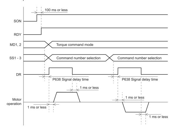
Figure 5-3 Internal torque command time chart
