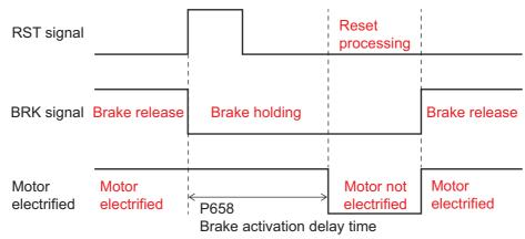
After the elapse of the time that is set in [P658 (8th - 5th digits)] from an ON edge of the reset signal (RST), reset processing is performed.
