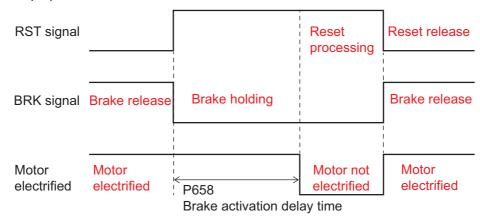
④ If the reset signal (RST) is turned ON (if it is held ON for a time shorter than the [P658 (8th - 5th digits)] setting)
