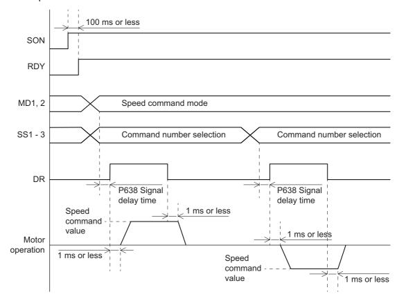
Figure 5-1 Internal speed command time chart
