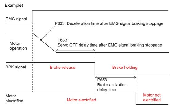
\* In the case of coasting to stop ([P633 (1st digit)] = Servo OFF), the motor operates as described in ① or ② above.
