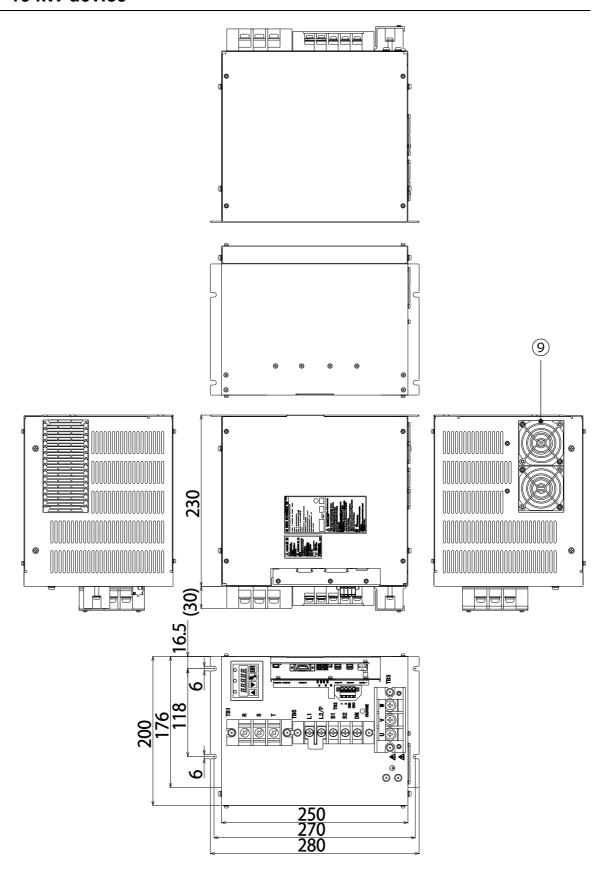
Figure 13-11 Outline drawing of the main unit of the device with 15 kW (Type 6)
