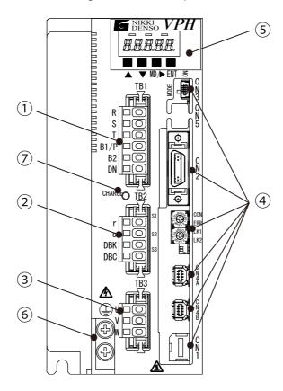
Figure 13-4 Front view of the main unit of the device with 800 W (Type2)
