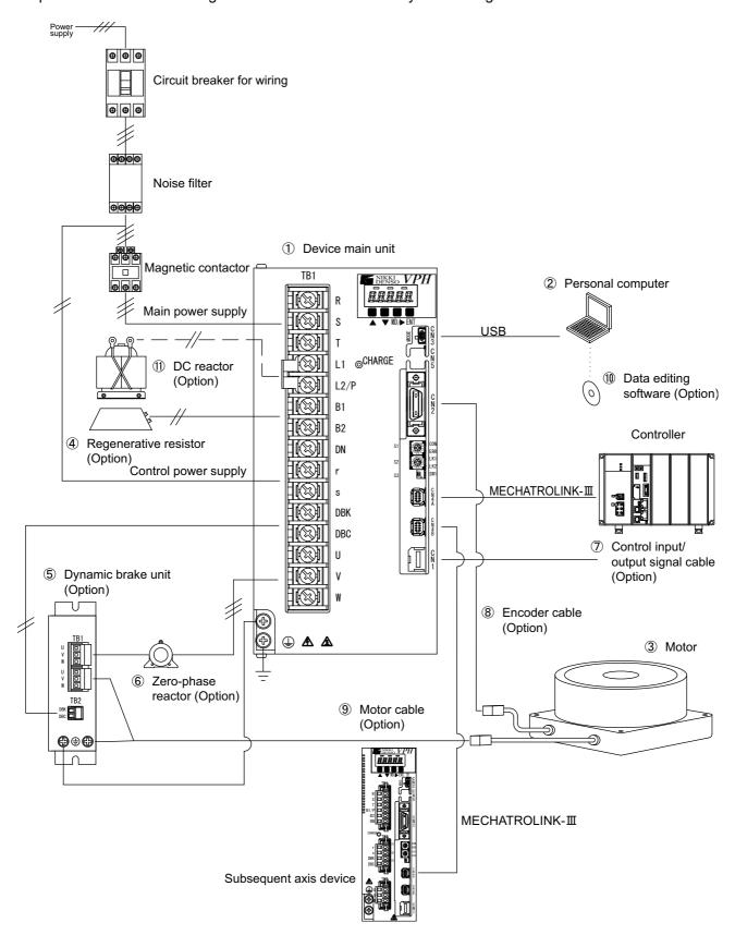
Figure 1-2 VPH HE Type system configuration for the 1.5 kW class or more
