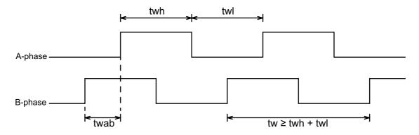
When [P140 (4th digit): Pulse output effective selection] is set to [1: Effective], these encoder pulse outputs function.
