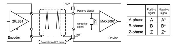
• Be sure that encoder feedback pulse is line driver (26LS31 equivalent) output.
