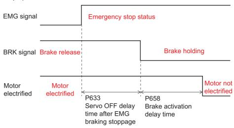
⑥ When a torque free alarm and a warning occurs If a torque free alarm or a warning occurs, the brake holding status is assumed and the motor is un-electrified at the time of its occurrence.
