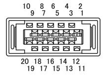
For pins 13 to 18, one of the following specifications can be set with [P140(4th digit): Magnetic pole sensor signal pulse output selection].
