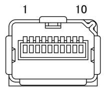
Table 3-1 Control input/output connector pin alignment
