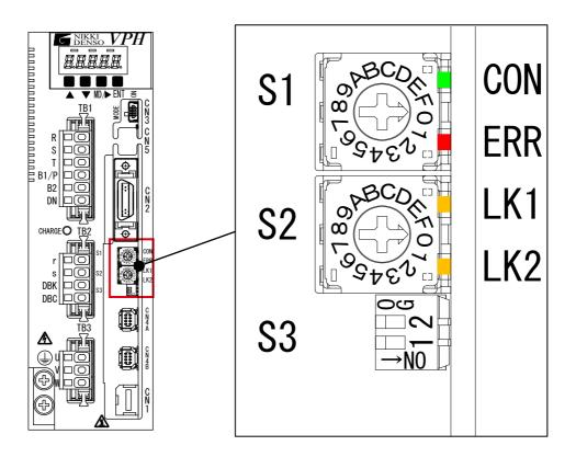
Figure 1-3 Setting a station address
