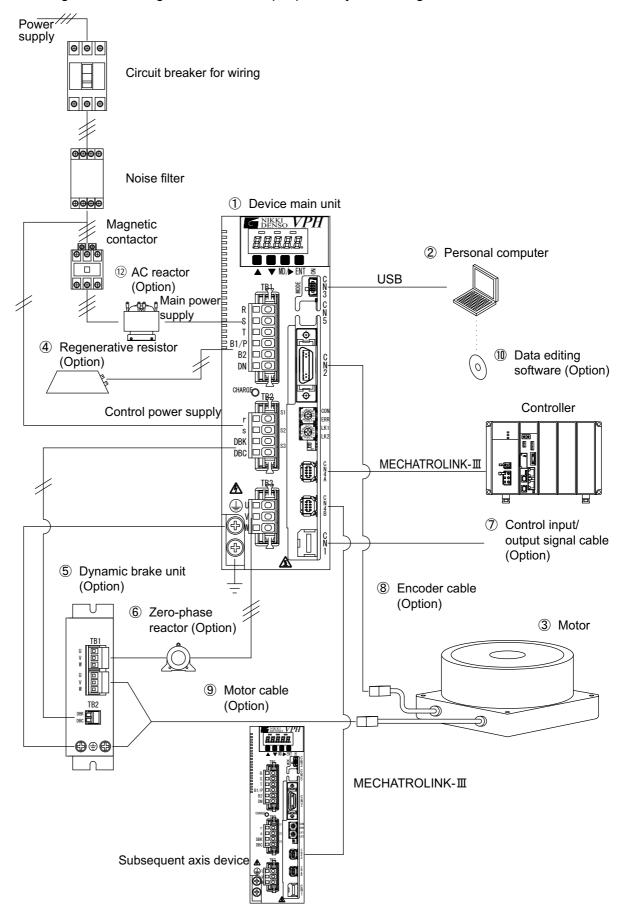
Figure 1-1 VPH HE Type system configuration for the 800 W class or less
