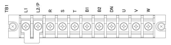
Connect the grounding to the grounding terminal on the device cabinet. When not using a DC reactor, do not remove the shorting bar between L1 and L2/P.
