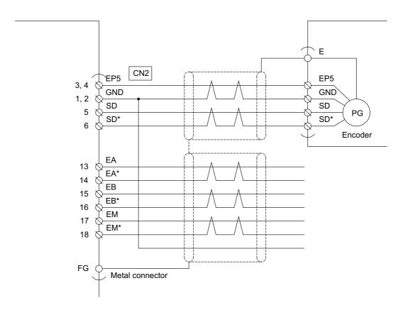
Figure 3-2 Serial encoder connecting diagram
