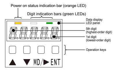
Figure 12-1 Configuration of the operation panel
