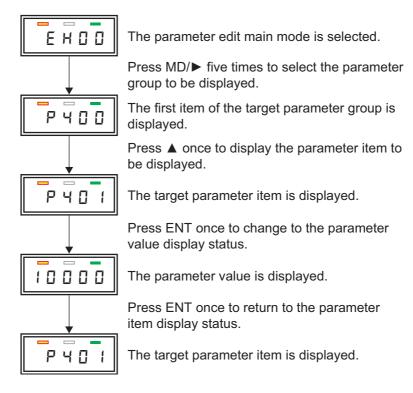
Figure 12-5 Example of displaying P401 data
