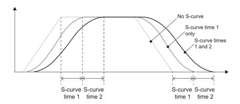
Figure 5-7 S-curve acceleration/deceleration operation example
