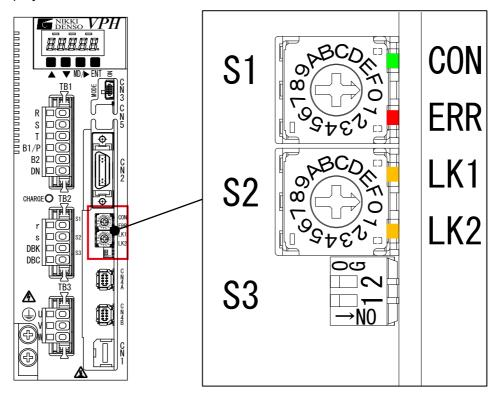
Figure 1-4 Appearance of the communication status display LED panel
