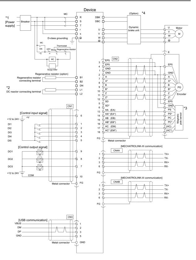
Figure 3-1 External wiring diagram
