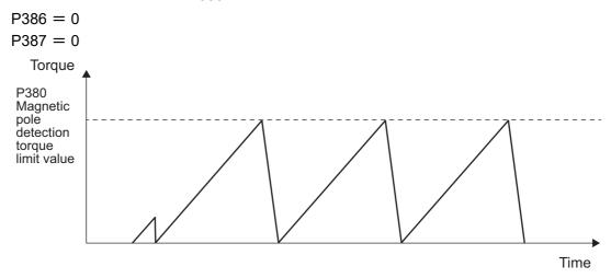
• Example 2: If the load inertia is equal to or greater than several tens of times the motor inertia
