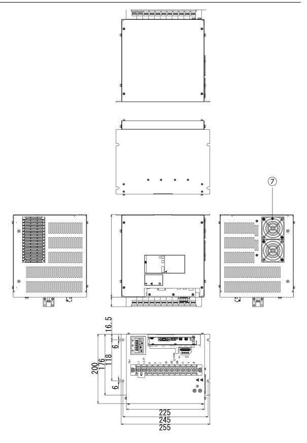
Figure 13-9 Outline drawing of the main unit of the device with 200 V and 7 kW (Type 5)
